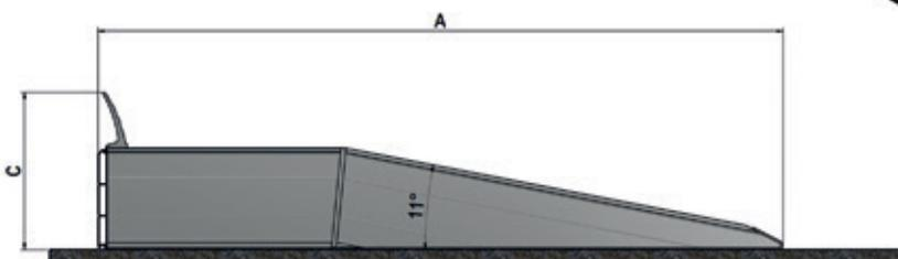
Definitive CLM offers wedges for lifting vehicles, they bring the floor of the van up to the level of the loading and unloading docks of logistics warehouses, in order to facilitate and ensure the safety of loading and unloading operations, and thereby speed up the entire process.
